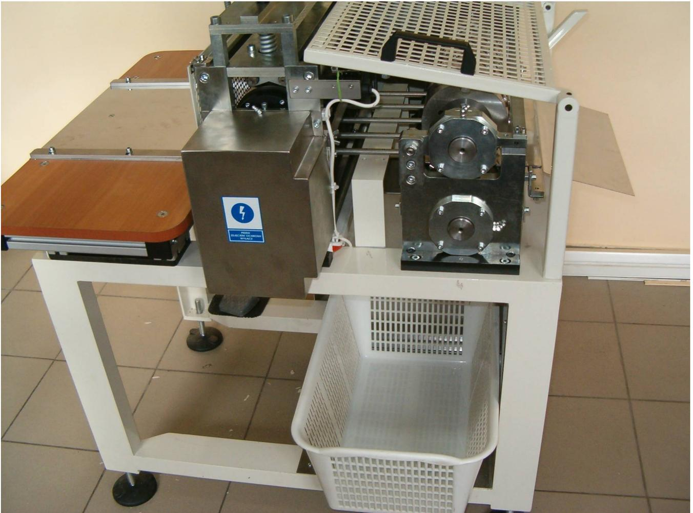
All components of K-35 placed on self-supporting steel frame covered by protections. All machine elements having direct contact with product are made of materials approved by the State Institute of Hygiene (PZH).
