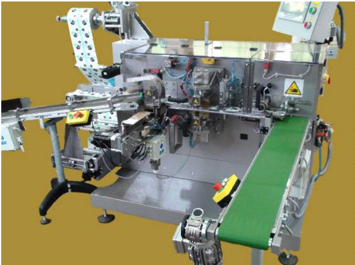
Very useful machine for packing pyramid teabags into heat sealed envelope, Then you pack flavoured and good quality tea blends, aromatic herbs or pharmaceutical infusion you are in a position to protect aroma thanks to heat sealed outer envelope.
